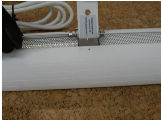
Dismount a bracket of the heater
